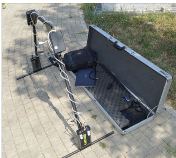
Slika 8. Georadar EasyRad Ground Penetrating Radar (GPR)
