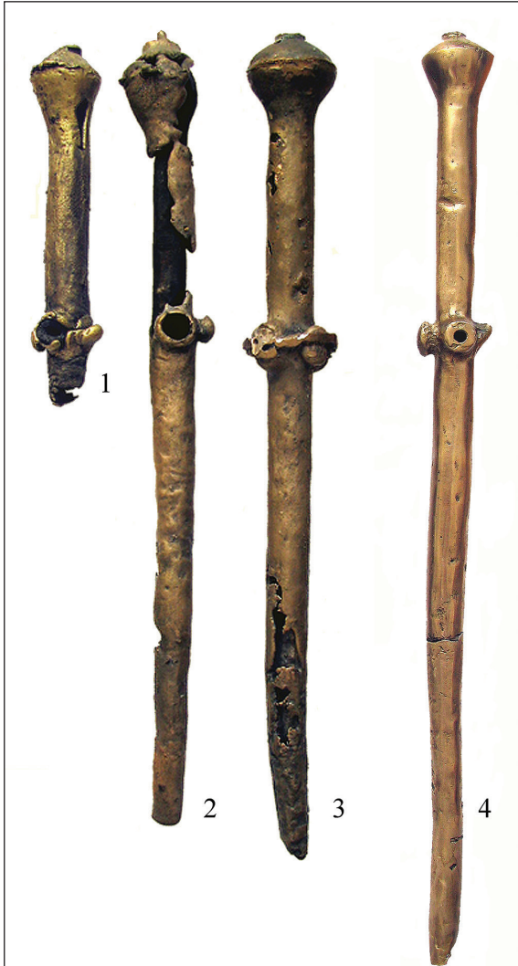
Fig. 8. Experimental castings. 1–3 – misruns in the casting; 4 – the final hollow casting.
